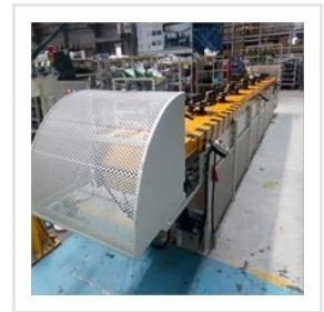
Slat Conveyor For Radiator Assembly
