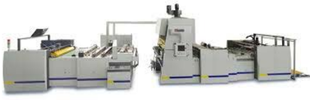
Typical Dry Lamination m/c using Water based Adhesives
