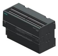
SIMATIC S7-200 SMART CPU CR60s, COMPACT CPU, AC/DC/RELAY, ONBOARD I/O: 36 DI 24V DC; 24DO RELAY 2A; POWER SUPPLY: AC, 85 - 264 V AC AT 47 - 63 HZ, PROGRAM/DATA MEMORY: 20 KB
