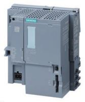
SIMATIC DP, CPU 1514SP-2 PN for ET 200SP, central processing unit with work memory 600 KB for program and 3.5 MB for data, 1st interface: PROFINET IRT with 2-port switch, 2nd interface: PROFINET RT, 6 ns bit performance, SIMATIC Memory Card required, BusAdapter required for 1st interface
