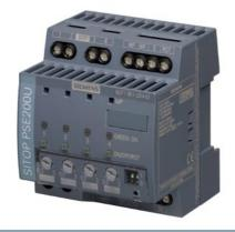
SITOP PSE200U 3 A NEC CLASS 2 selectivity module 4-channel input: 24 V DC/12 A output: 24 V/4x 3 A NEC class 2 threshold value adjustable 0.5-3 A with status message for each output
