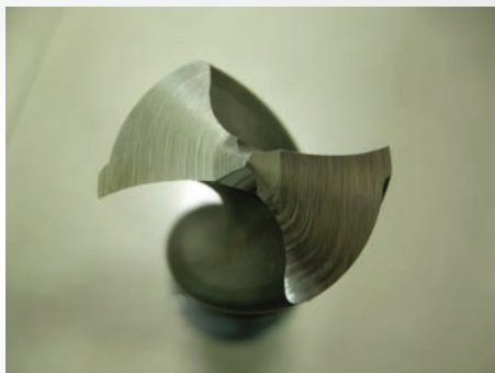
\varnothing 40\text{ mm} drill bit (after re-sharpening)
