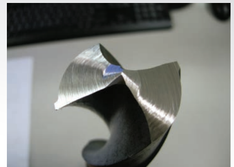
\varnothing 50\text{ mm} drill bit (after re-sharpening)
