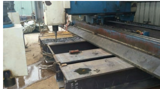
Hang type, H-Beam drilling
