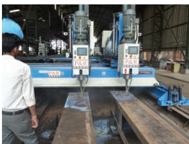
Rail type, H-Beam drilling
