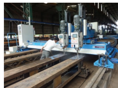
Rail type, H-Beam drilling
