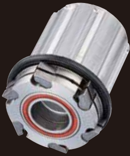
R07-G2C2 Titanium Shimano 11s Weight : 111g Material : Titanium Bearings : 3 (6802*2+6902*1)
