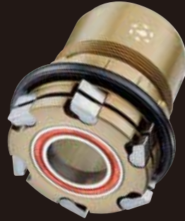
R07-D2C2 Alloy SRAM XX1 Weight : 73.4g Material : Alloy Bearings : 2 (6802*1+6902*1)
