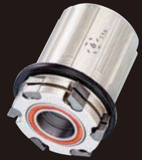
R07-K2A2 Steel Shimano 11s For BX103R Heavy Duty Weight : 153.8g Material : Steel Bearings : 3 (6802*2+6902*1)
