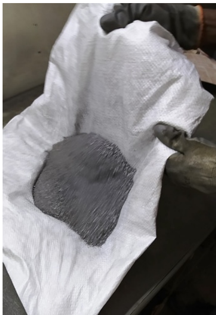
Total 7 kgs (- 10 MM) further crushed to -2.0 MM mixed up properly.
