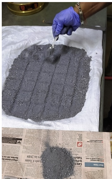
Sample size reduced to 400 gm by I.R. Method (3 stages)
