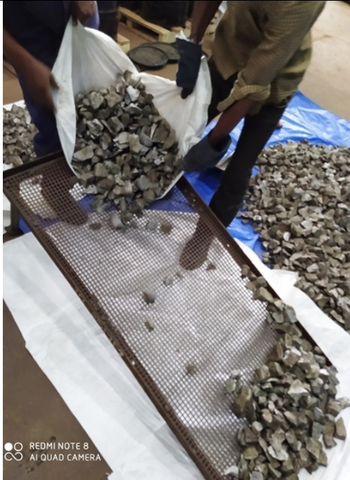
Sieving in progress to check material below 10 MM size in progress
