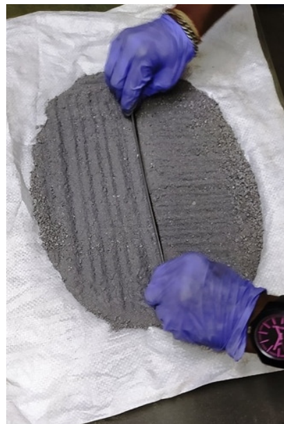
Sample spread uniformly for I.R.
