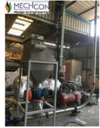
Vacuum Dilute Conveying System
