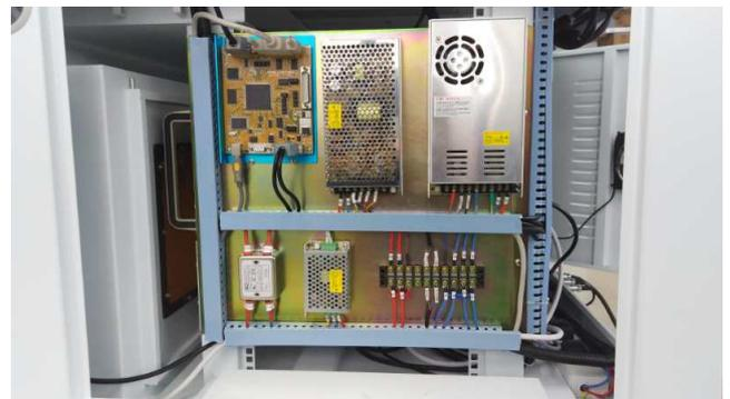
1. Three laser supply independent supply galvo laser source control card avoid mutual electric interference.
