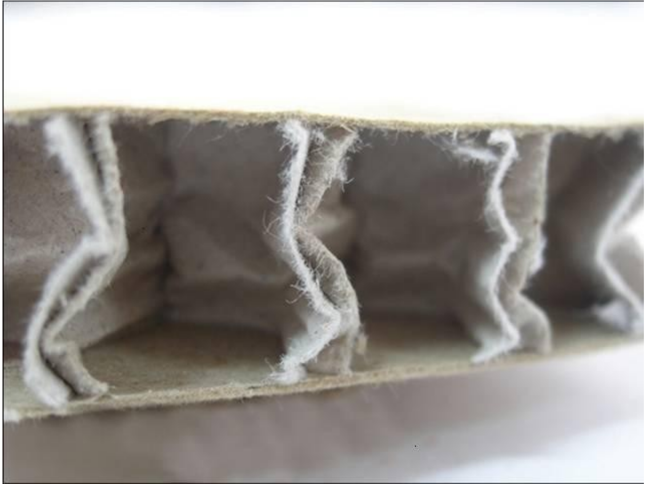
The honeycomb cardboard flat compression deformation of specimen
