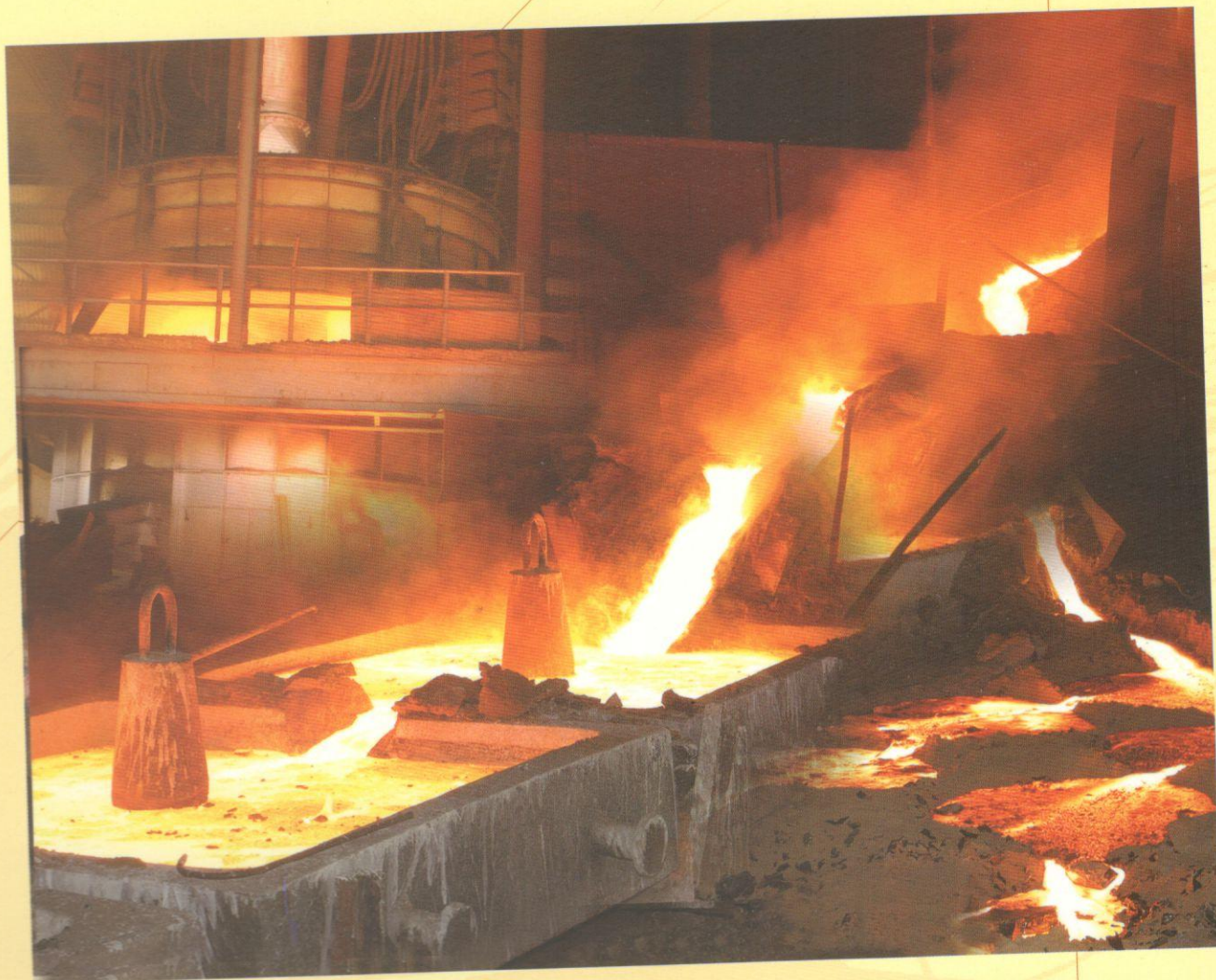
Continuous tapping of Ferro Alloys in Submerged ARC Furnace
