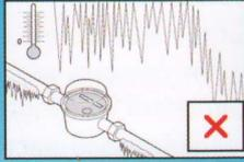
Water meters should never be installed where there is a risk of water ingress, for example, underground or exposed to the elements at any time. Additionally, they should not be exposed to extremes of temperature. Like any other fitting, freezing / heating can damage the dial mechanism and crack the meter body. Meters should always be protected from these risks.
