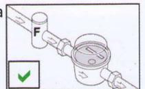
5. Only clean water should be used that does not exceed the temperature specification of the water meter. [Temperature specification is 45°C for COLD Water Meters and 90°C HOT Water Meters.]
