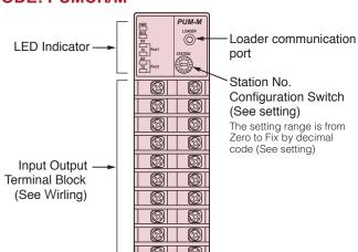
**LEDindicator** Six LED lamps indicate the following operational conditions
