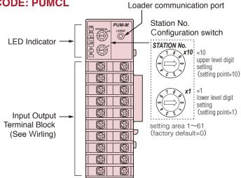
**LEDindicator** Six LED lamps indicate the following operational conditions
