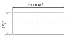
Note: When panel mounting, two bracket are necessary either on the top and bottom of the recorder.
