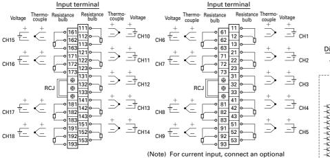
shunt resistance to a voltage input terminal
