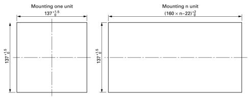
Do not use the water proof packing in case of mounting  $\boldsymbol{n}$  unit
