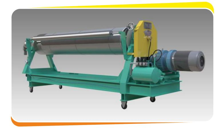
Technical details:-Vacuum unit roll diameter: - 480mm Main frame size: - 3000 mm x 750 mm x 1200 mm Maximum speed: - 25 m/min
