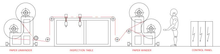
As an organization we ensure that our design and engineering stay ahead of our clients demands. After production of artificial leather needs to inspection properly so we do universal inspection table for it. Our inspection table maintains uniform tension control system. Full forward & reverse batch roll take off system are provided. Electronic length counter meter supplied for measuring lengths such as production counting of finished product.
