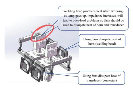
The better the heat-dissipating effect is more stability the continuously work
