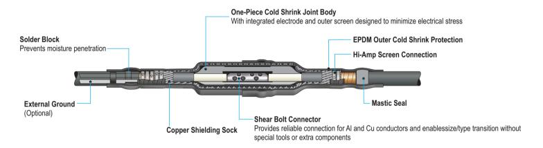
Easy, consistent installations by eliminating the pushing, pulling or heating required by traditional splices silicone rubber body which provides excellent electrical properties and superior low temperature handling.
